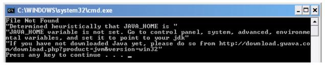
Save, and run the install. The server MUST have internet access for this installation to work. After the installation has completed, specify the JAVA\_HOME variable.
