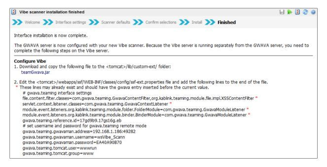
After the Vibe interface has been installed, follow the ending instructions for both local and remote installations. Remote installations will require manual editing of the Tomcat files, as the interface wizard will not have access to them during install. Input the specified lines around the indicated, existing lines in the ssf-ext.properties file, so the file section matches the one shown.
