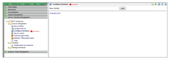
The default domain specified during Server Activation will be specified. Additional domains may be added through the new domain addition field along the top of the screen. As always, make sure you save all desired changes made to the page before browsing to a different section of the management console.
