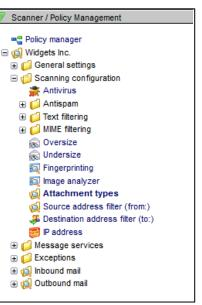
The example now shows the attachment type scanning enabled and the inheritance forced to prevent accidental disabling of the service later on.
