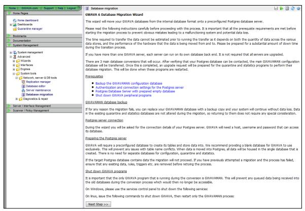
Shutting down all peripheral programs to gwava, except the 'gwavaman' process will leave the administration interface functional and accessible for the migration process. It is critical that all peripheral GWAVA process be shut down before the migration is started.
