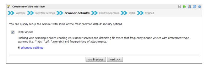
Select the scanning options and configuration for the interface. The interface settings may be changed after the interface is created, and defaults show the blocking of viruses and spam.
