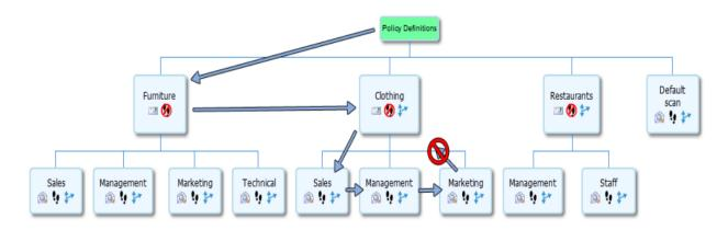
Backtracking is a feature that is normally wanted for the very purpose of falling back to a default scanner, however when you come across a need to stop a specific type of mail from being scanned, backtracking provides that ability.
