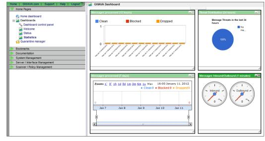
The statistics dashboard contains basic statistics for the entire system with all interface stats available to be monitored. The statistics vary from total messages processed in the system and breakdowns of different blocked messages to the number of operational threads and system loads according to time of day.
